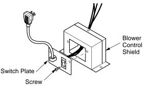
Figure 17 - Installing Switch Plate to Blower Control Shield
